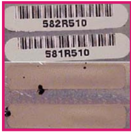
FIGURE 6: Two polyimide labels, exposed side-by-side at 600°F (312°C) for 50 minutes. The label at top performed satisfactorily, while the label at bottom became discolored.
