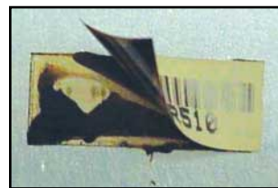
Figure 3. Photograph of polyimide label subjected to 300 °C for 50 min.
