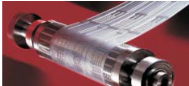
Figure 1: For many label manufacturers the magnetic cylinder die-cutting technology paved the way from flat-bed to rotary die-cutting.
