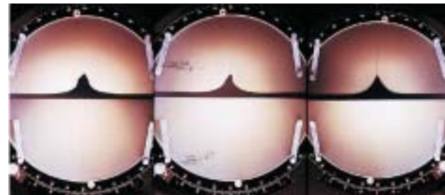
Figure 3: These three variations are of limited use for faultless die-cutting. Left: a manually sharpened profile with visible weaknesses at the different angles. Middle: Etched profile partly manually equalised. Right: Mechanically sharpened cutting edge of earlier days.
